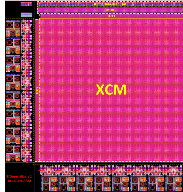
Layout Floorplan of the Cross-Correlator ASIC
